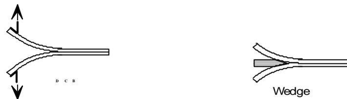
Fig. 2 DCB and wedge test methods
